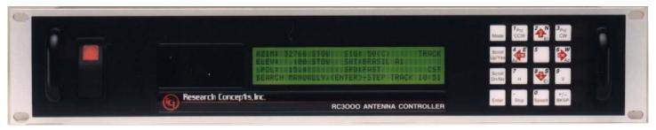
Avoid the time consuming tasks of manually positioning your mobile antenna and tracking inclined orbit satellites. The RC3000 allows even non-technical personnel to automatically locate and position a mobile antenna within minutes from power up.
