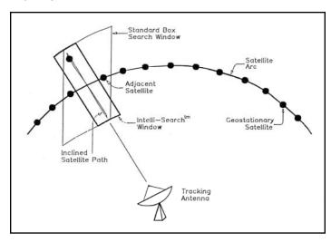
coincides with the satellite's expected path. Once an inclined satellite has been stored in the RC2000C, finding it again is as easy as locating a fixed satellite. Simply move to Auto mode, select the satellite from the list of those available, specify the proper polarization, and let the RC2000C do the rest.
