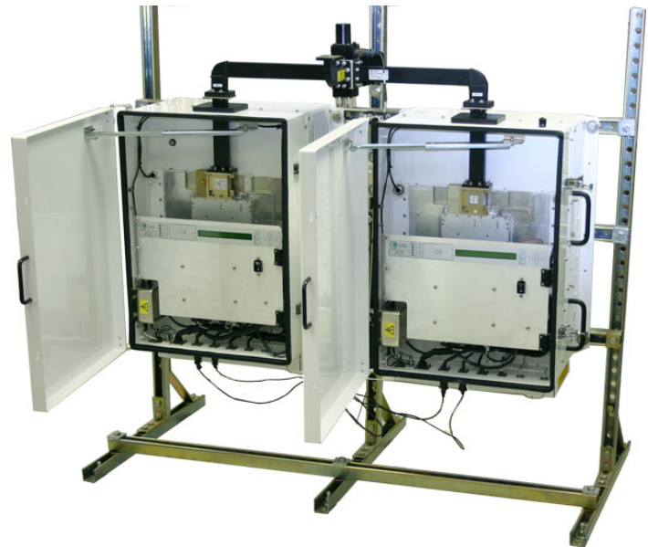
600W C-Band High Power Outdoor 1:1 Redundant System
