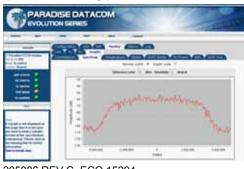
Simple to use BER Tester Option allows real time bit error measurements through traffic or ESC channel.
