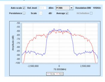
Built-in Paired Carrier web graph showing both of the overlapped carriers.
