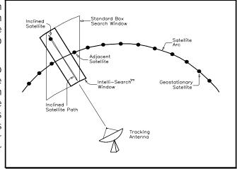
**SEARCH** is entered when the satellite signal has been lost. The RC3000
