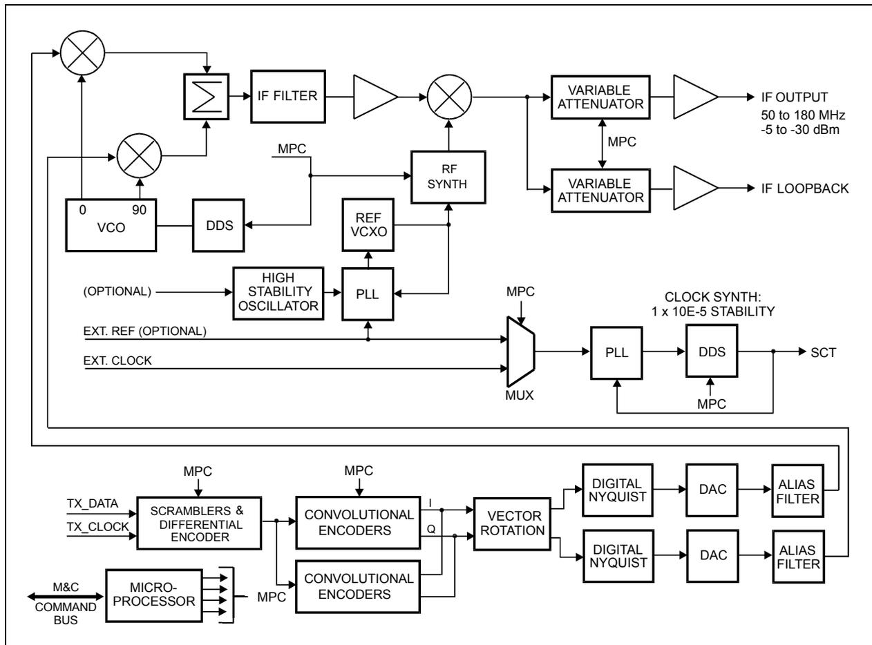
Figure 5-2. Modulator Block Diagram
