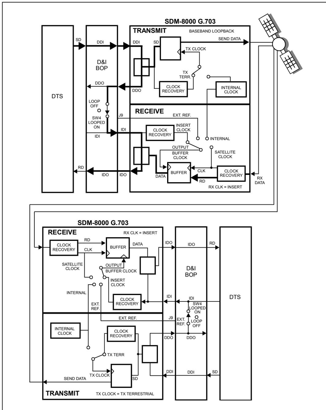
**Figure 6-7. Baseband Loopback (with D&I)**
