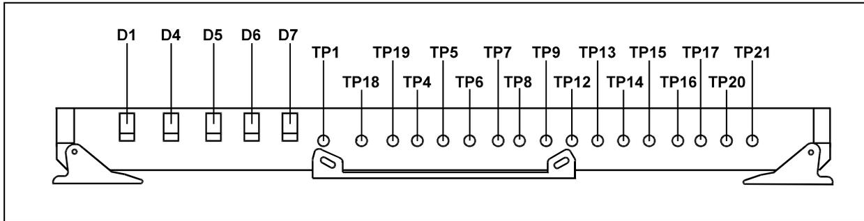
Figure 9-5. Interface PCB Test Points
