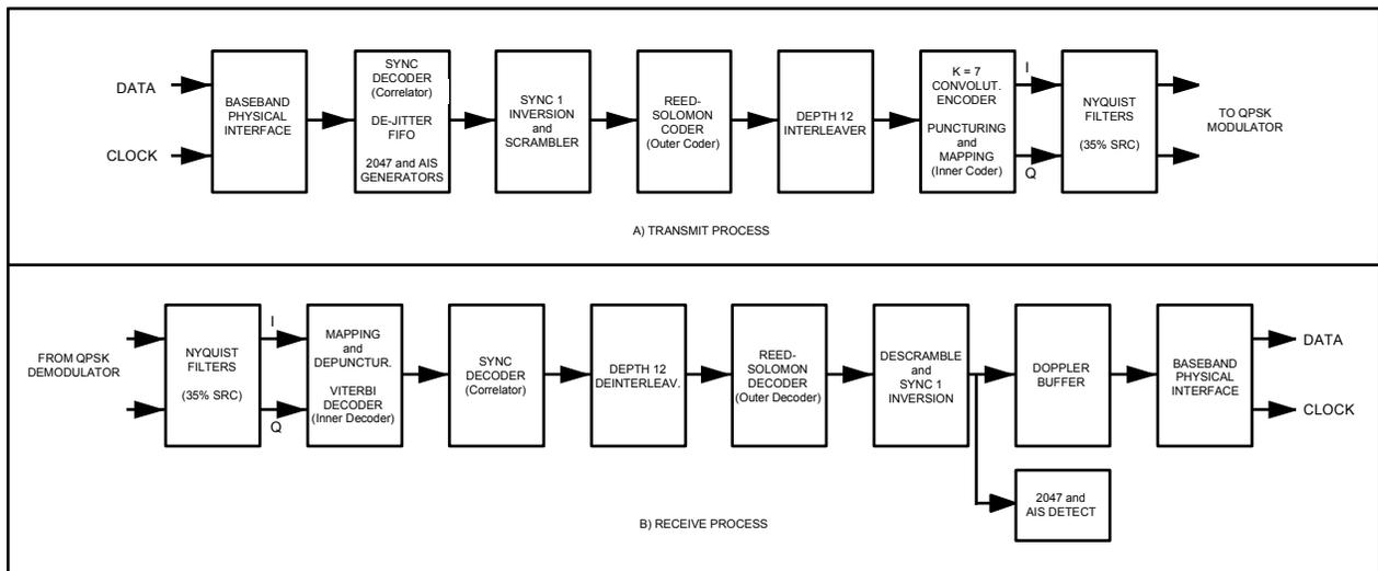
**Figure B-12. Block Diagram of SDM-8000 Configured for DVB Operation**
