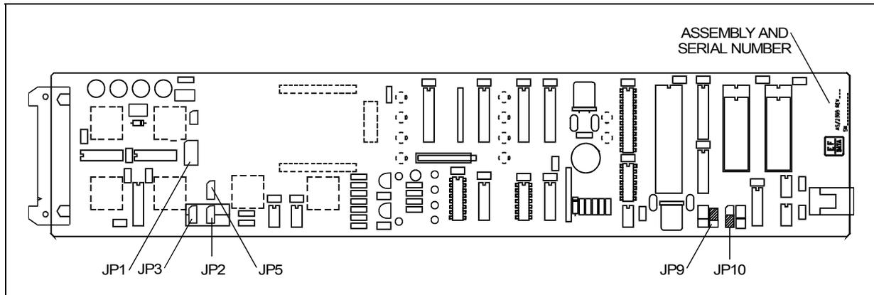
**Figure 4-1. Display/M&C PCB**
