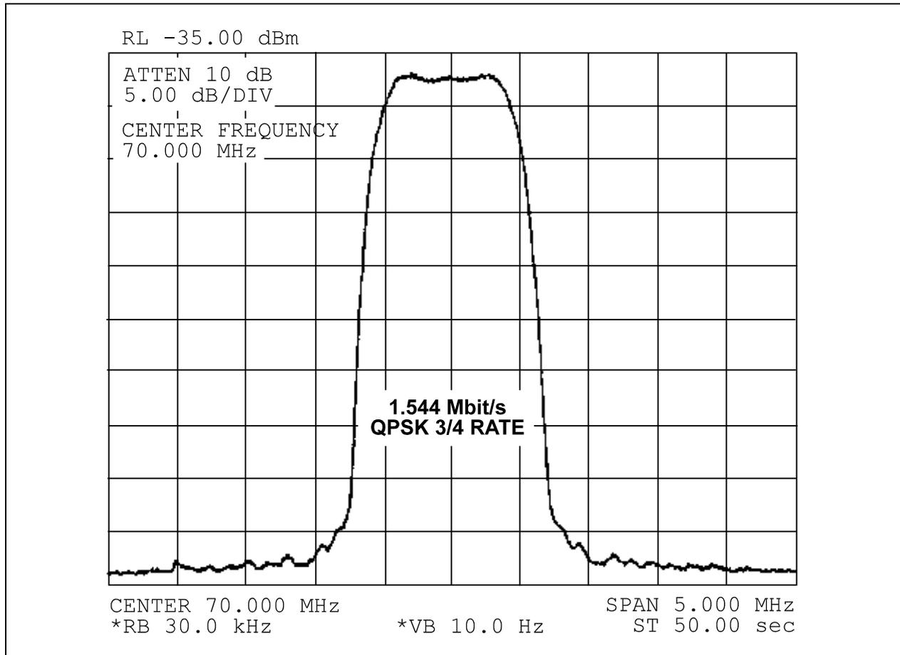
**Figure C-8. SDM-8000 Typical Spectral Occupancy**
