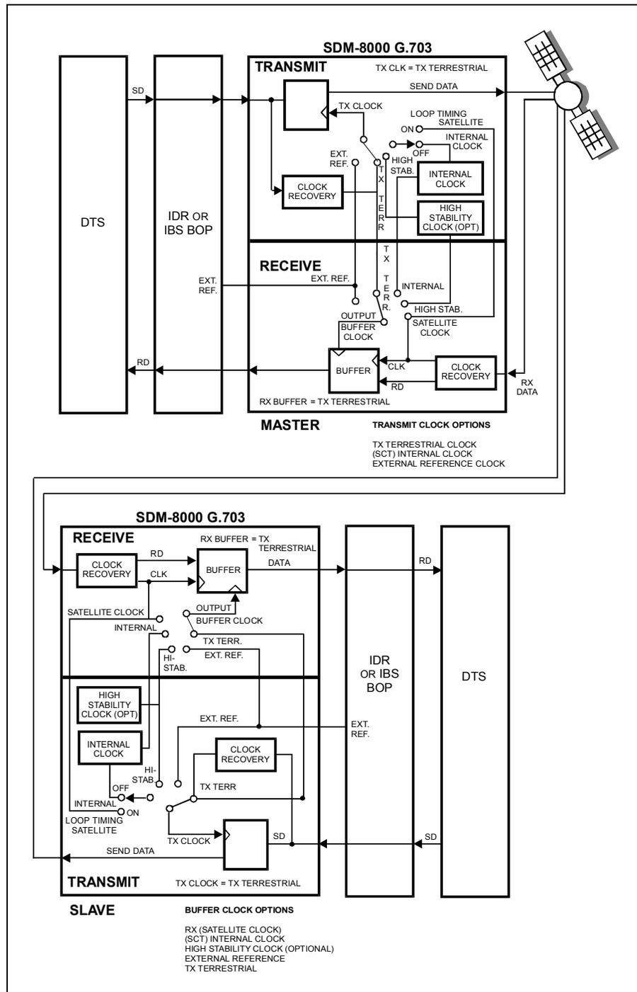
Figure 7-1. IDR/IBS G.703 Master/Master Clocking Diagram
