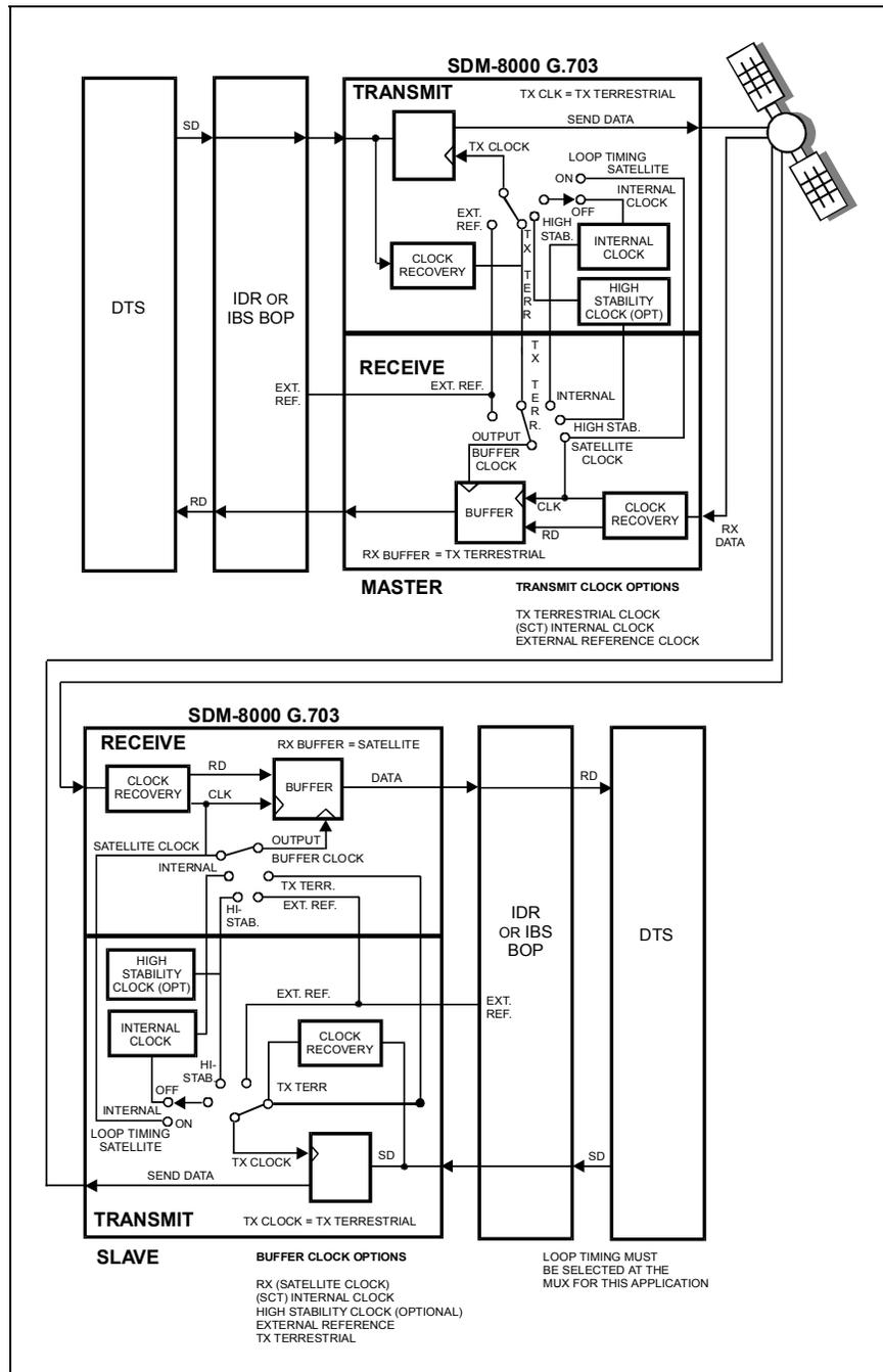
Figure 7-2. IDR/IBS G.703 Master/Slave Clocking Diagram
