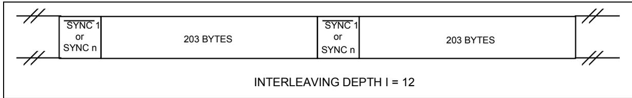
**Figure B-22. Interleaved Frame Structure**
