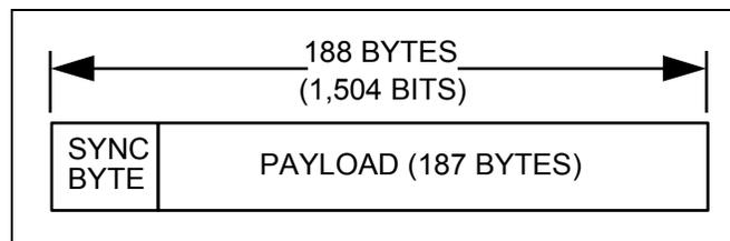
**Figure B-15. MPEG-2 Transport Packet**
