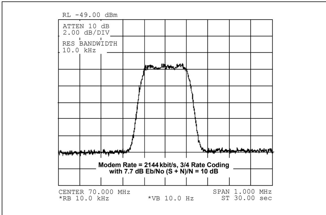
Figure 9-2. Typical Output Spectrum (with Noise)
