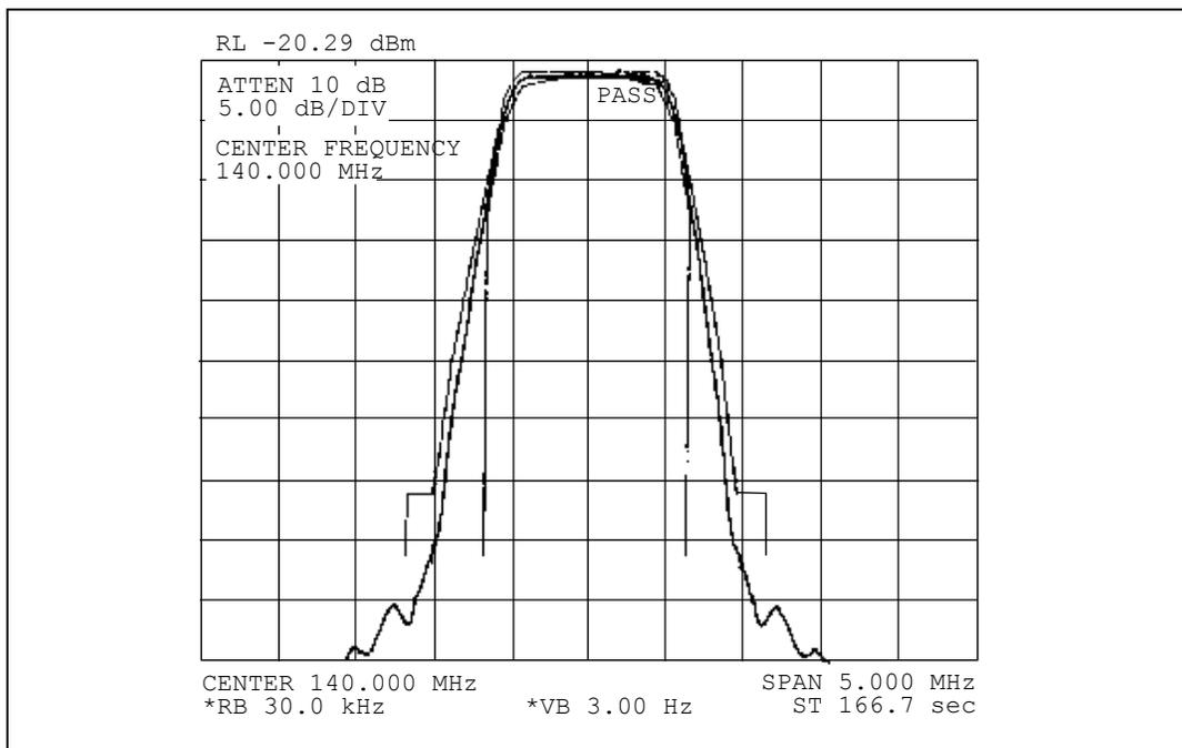
Figure 9-3. Typical Output Spectrum
