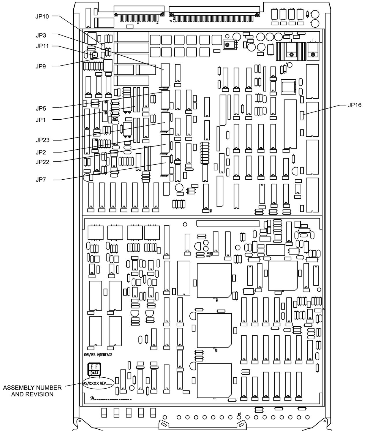
Figure 4-4. Interface PCB
