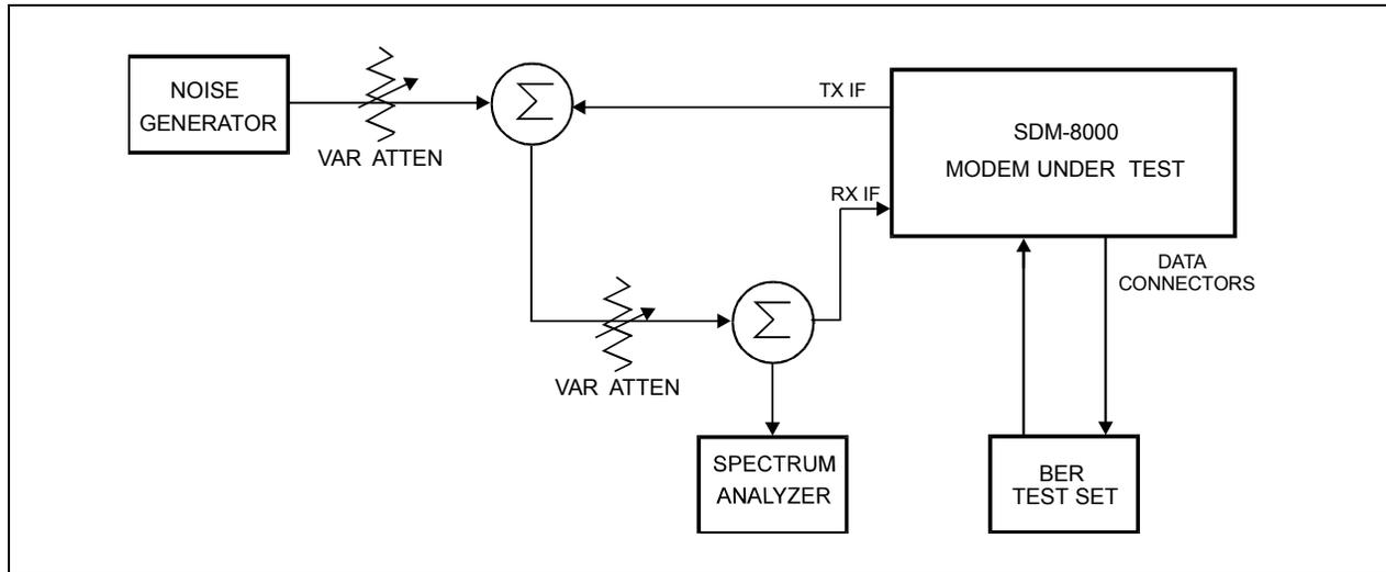
**Figure 9-1. Fault Isolation Test Setup**
