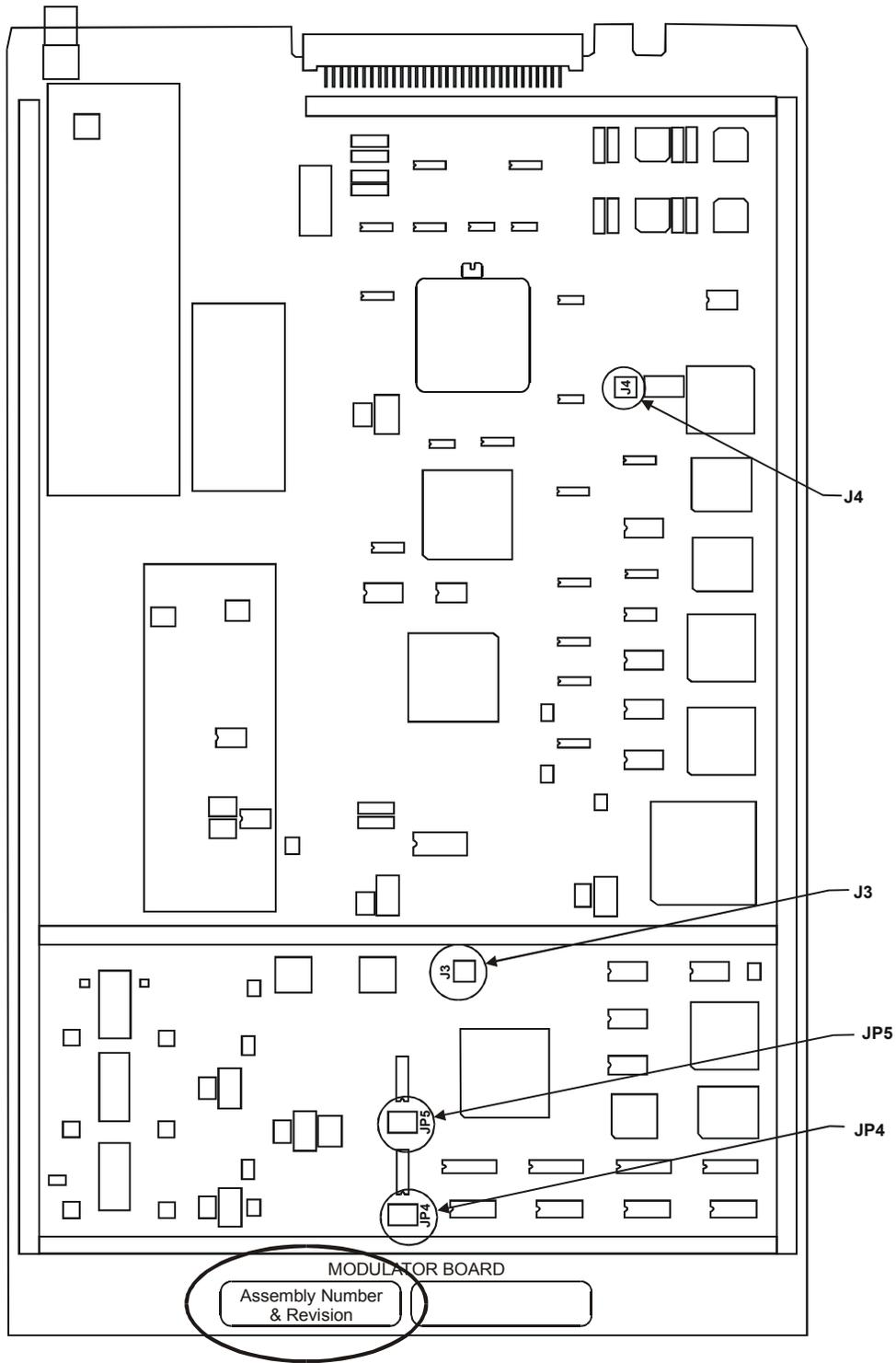
**Figure 4-2. Modulator (AS/5039) PCB**
