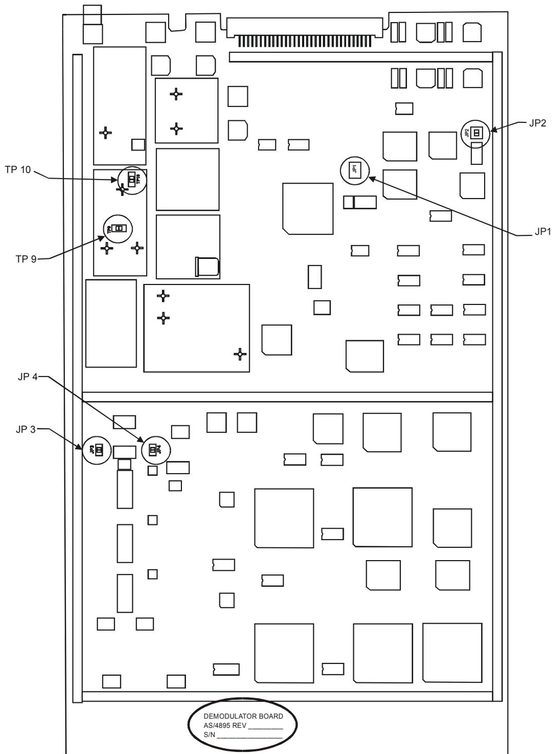
Figure 4-3. Demodulator (AS/4895) PCB
