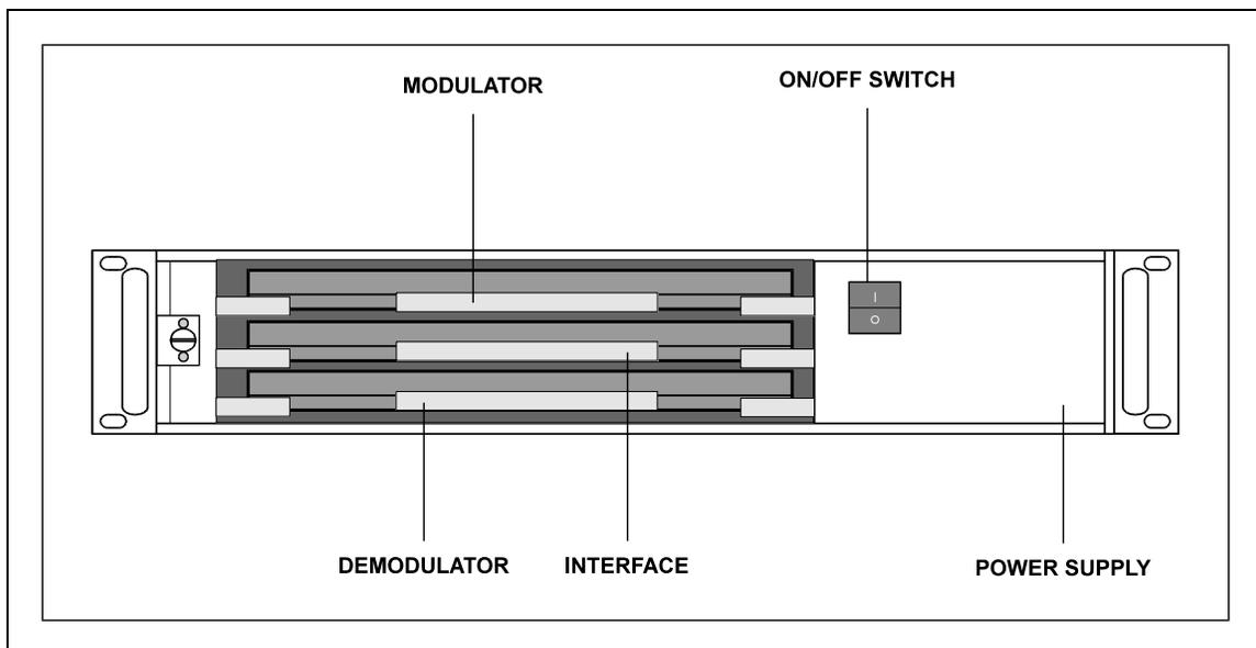
Figure 1-2. Modem Construction
