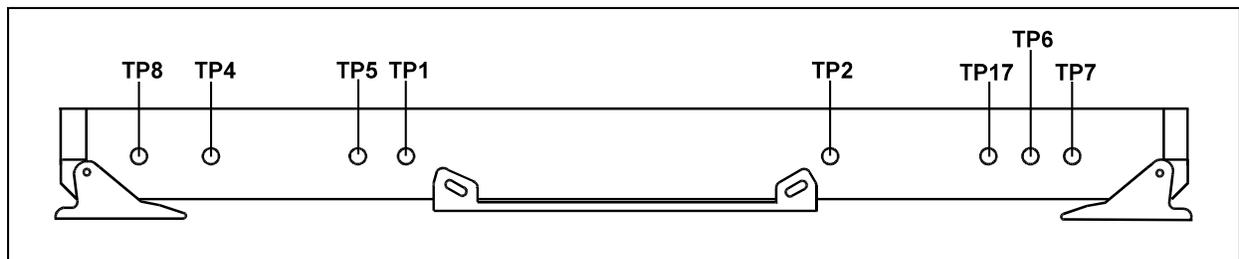
Figure 9-6. Modulator PCB Test Points
