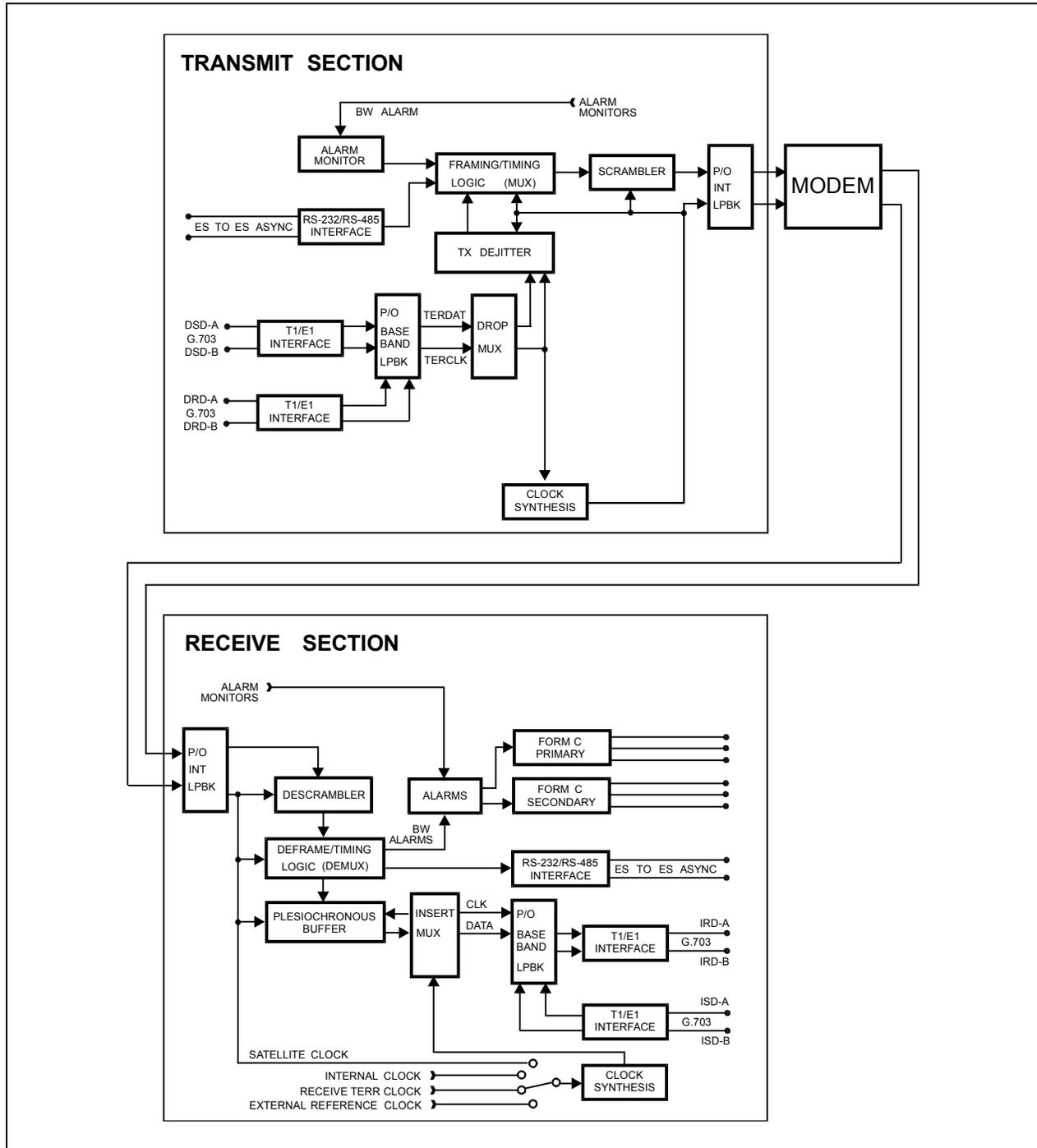
Figure B-3. D&I with Asynchronous Overhead Block Diagram
