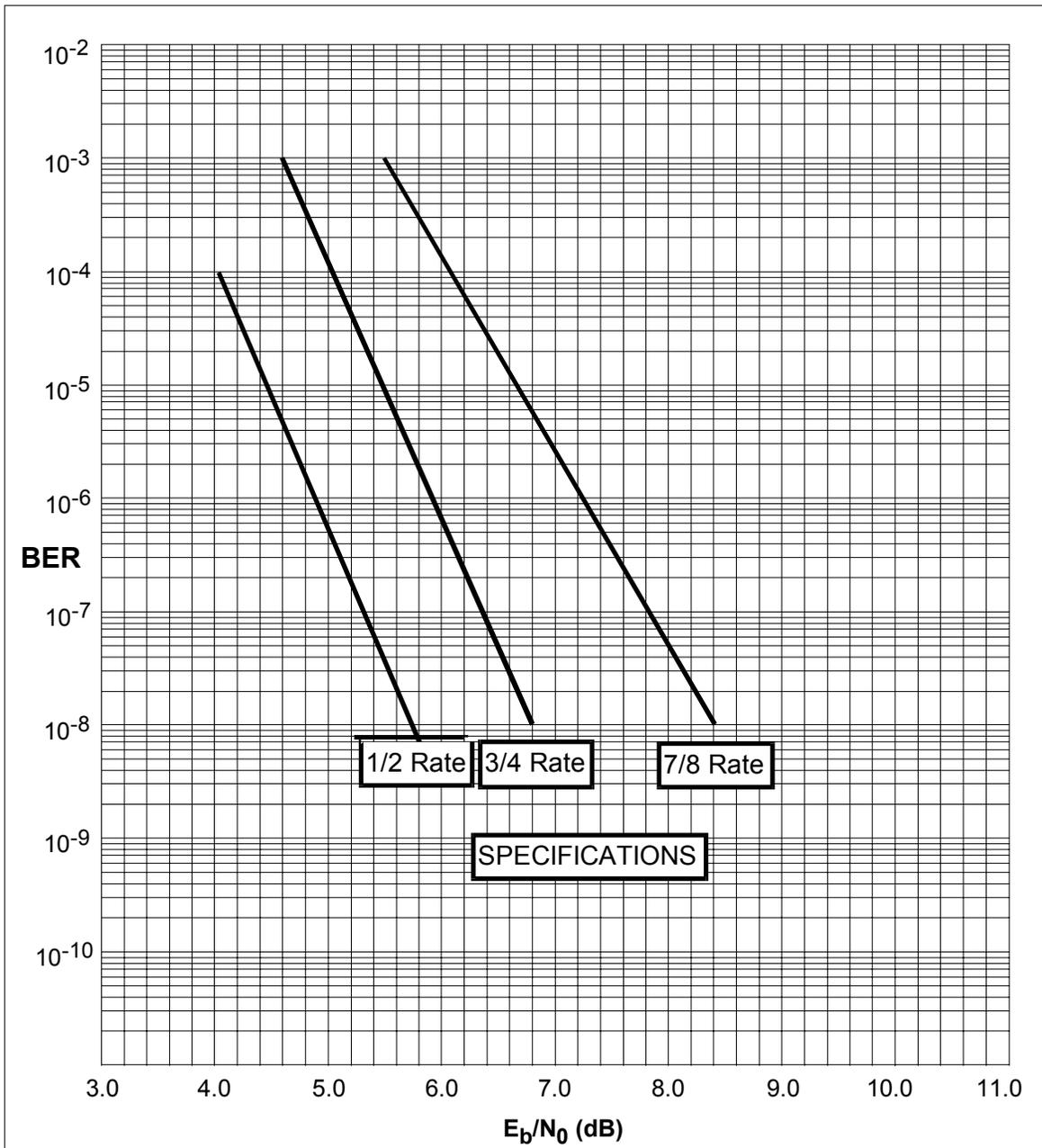
Figure C-2. Sequential Decoder 56 kbps BER Performance Curves
