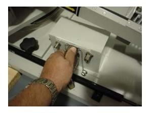
Remove all cables from the antenna pedestal.
