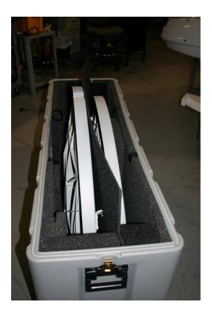
Re-insert the reflector halves into the equipment case, keeping the sections separated with the insulation material built into the case.
