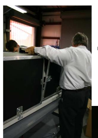
Re-secure all latches holding the cover to the pedestal.
