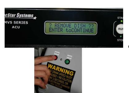
From the REMOVE DISH screen on the controller display, press the ENTER button. The pedestal will resume stowing.
