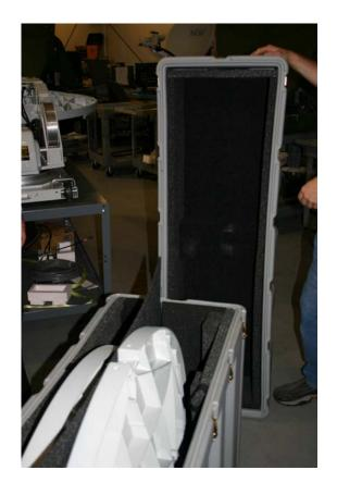
Open latches and remove the cover from the reflector case.
