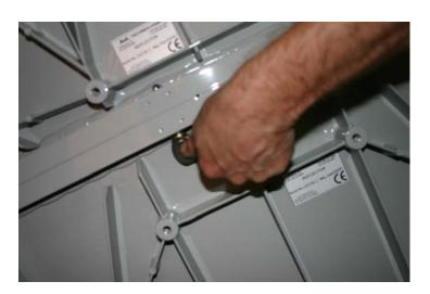
Open latches and secure the two reflector pieces together. Secure the reflector latches.
