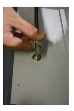
Remove the boom support struts from their position on each side of the pedestal base.
