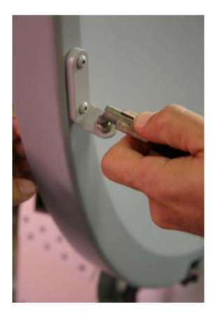
Lifting the end of the feed boom, remove the struts from the reflector and the feed boom ball studs on both sides of the reflector.
