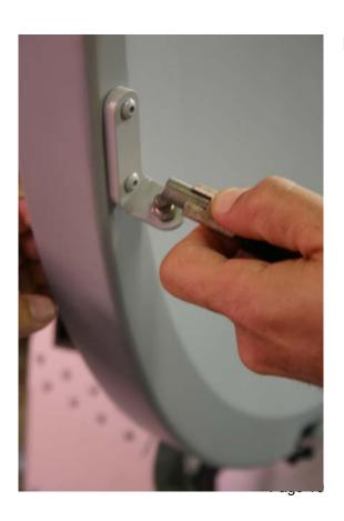
Lifting the end of the feed boom, secure the struts to the reflector and to the feed boom ball studs on both sides of the reflector.
