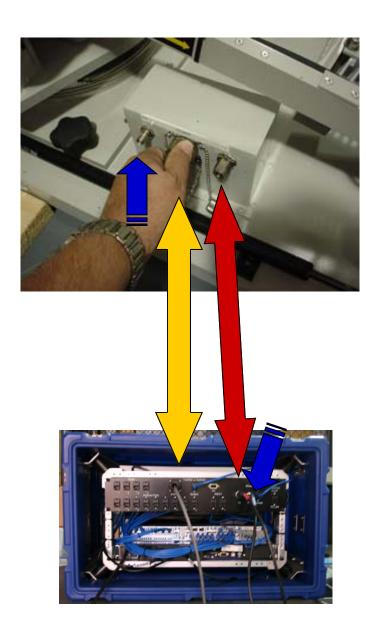
Connect the antenna controller cable to the antenna.
