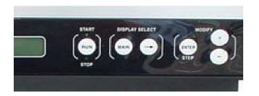
From the READY screen on the controller display, press the " + " button for 2 seconds. The pedestal will begin to lift.
