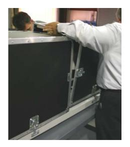
Open latches and remove protective cases from the pedestal.
